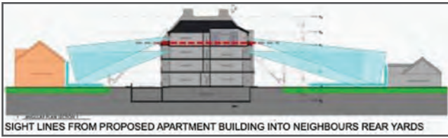
This shows the light that will shine into neighbouring homes, and the height of the apartment compared to nearby houses.
